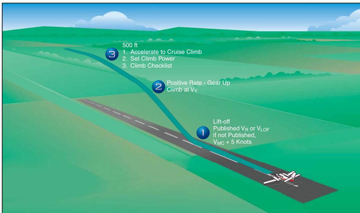
Figure 12-7. Takeoff and climb profile.
