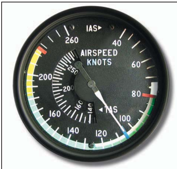
Figure 12-1. Airspeed indicator markings for a multiengine airplane.
